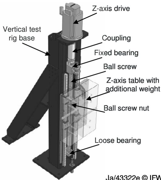
Figure 9: Experimental rig
