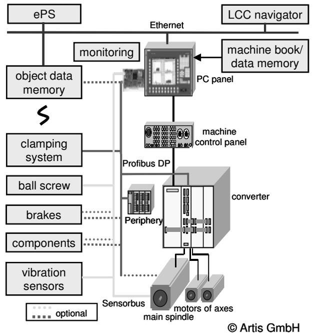
Figure 11: Concept for the life-cycle monitoring system
