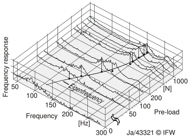
Figure 7: Eigenfrequency vs. pre-load
