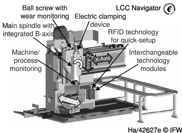
Figure 5: Model of the life-cycle oriented machine tool
